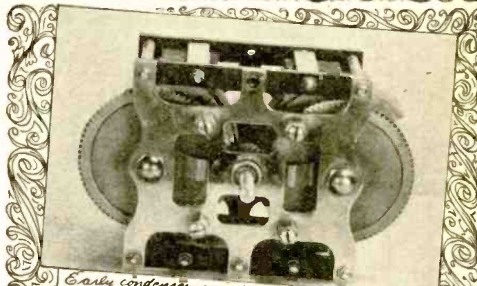
Early condenser-ganging by means of gears - 1925 G.I.C.
