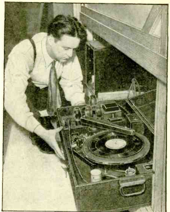
2 . . . INSTANTLY, an automatic electric phonograph starts up and the announcer's voice issues from the loudspeaker. "This exhibit," he begins and rambles on into an interesting discussion illustrated by changing scenes. On the recording, at intervals, are specially-cut grooves which actuate relays controlling the lights. Then . . .
