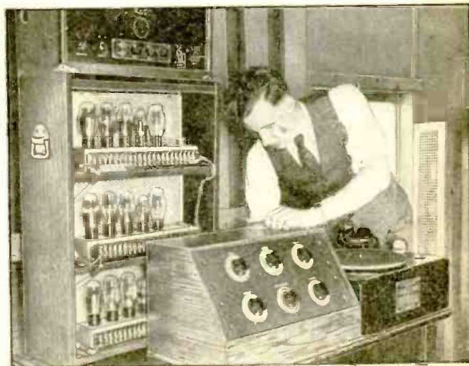
S TRANGE BAGGAGE IN THE BAGGAGE CAR! Note the phonograph and the mixing panel. By means of these controls the operator can "cut-in" the various microphones or switch-in the phonograph. The train's 32-volt lighting system operates the sound system's motor-generator set.
