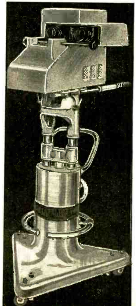
Fig. D. The new English Emission electronic television camera. It is used in a "television truck" for televising "spot" programs.
