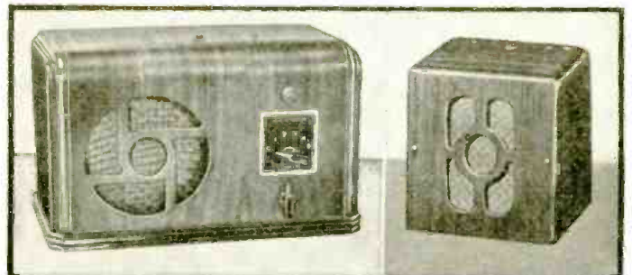
The Radolek Co. A selective A.F. system using a master unit and 1 to 5 outlying stations is the essential part of this interphone. The amplifier in the master unit contains 3 tubes—a 6C6, a 43 and 25Z5 for A.C.-D.C. power supply. Interconnecting cables are used between the master and outlying stations.
