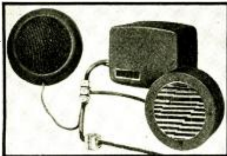
Zenith. Sensitivity, 0.9-microvolt; output, 9 W.
