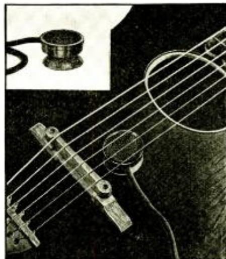
Fig. 1. An electronic pickup for converting musical instruments into electronic instruments. The "contact-type" microphone attaches to the instrument by means of a rubber suction cup (see inset).
