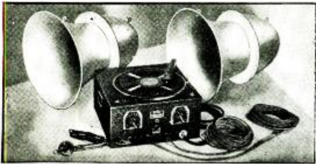
A 20-W., "beam"-type "campaign" sound system. (1188)
