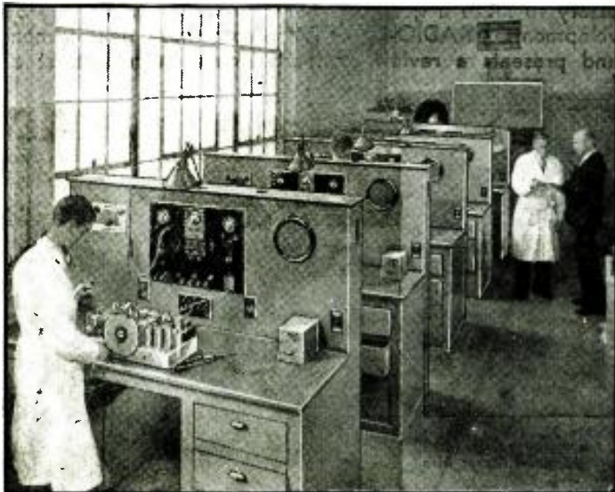
(Photo—Philco Radio & Television Co., San Francisco.) The modern service bench, with its test speaker, tube checker and set analyzer, is a model of efficiency. Above are shown 5 of them in a factory.
