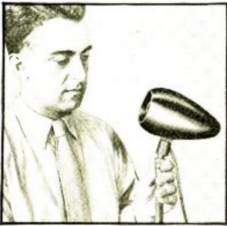
Fig. A. The neat appearance presented by the bullet mike is evident from this view. Because of the high efficiency, and directional characteristics "close talking" is not necessary.
