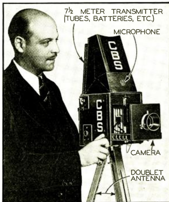
Fig. B. The "photo-mike," and its creator, E. K. Cohan, of CBS.
