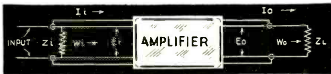
Fig. 1. The factors involved in db. gain and level.
