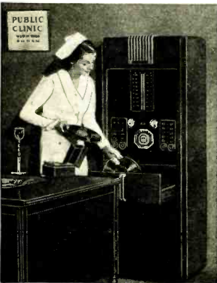
W. E. Co. Photo. A modern 2-channel hospital sound installation. It provides patients with radio-phono, entertainment. Unit also includes talk-back facilities—the speakers act as "mikes"; see page 688.
