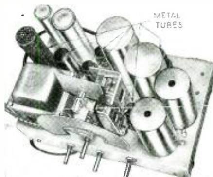
Below, the A63 metal-tube chassis.
