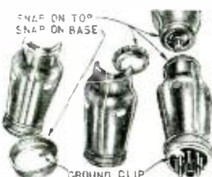
Above. Glass-'metal' tube shield. (820)
