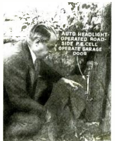
Fig. D, below Cleverly concealed PE. cell lights up grounds.
