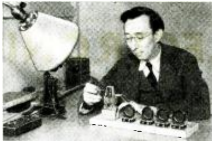
The appearance of the Hewlett sun motor which uses four selenium photo-cells.
