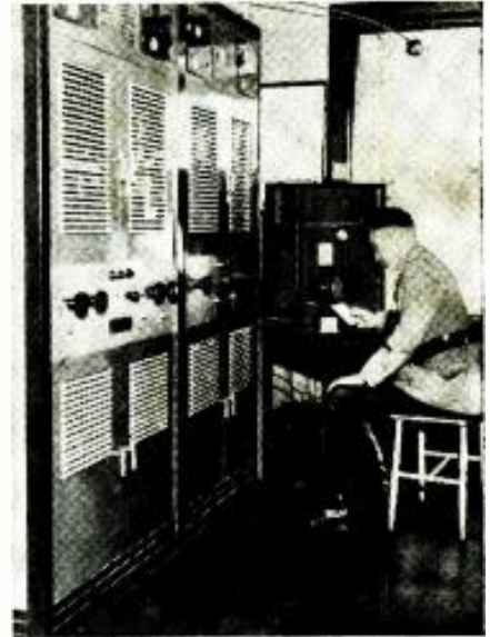
The new 1000 watt transmitter of the New Jersey state police—W3XCW.
