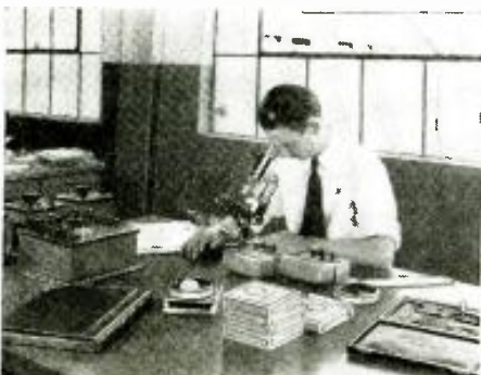
Filament and heater wire is critically examined before being accepted for radio tubes; its diameter is checked—its composition is examined microscopically for structural features.
