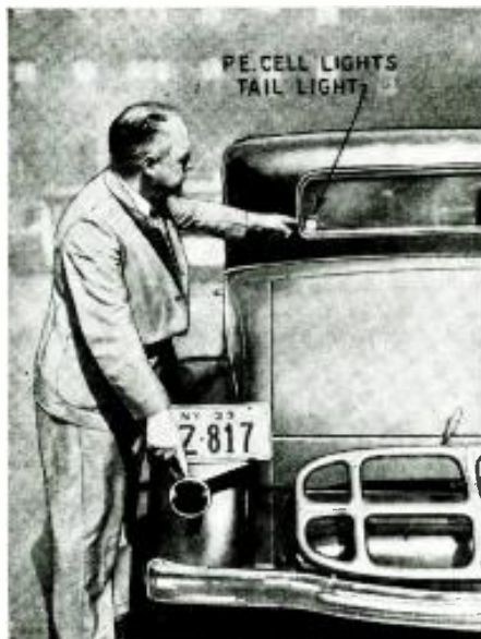
Fig. G.—PE cell turns on parking light.
