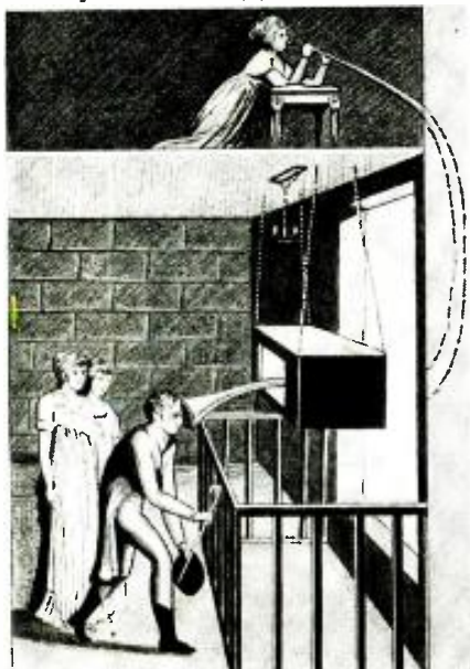
Fig. B The "mysterious box" or "invisible singer" combining the acoustical pipe and large horn.
