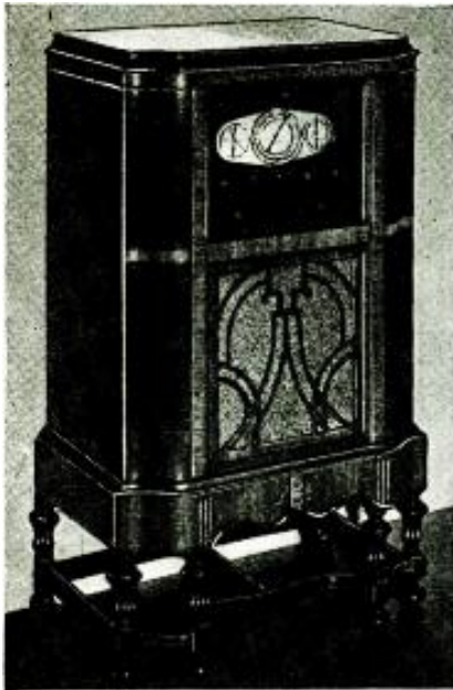
A 19 tube radio receiver in its home. Airplane-type dials are used; only the tuning dial sector of the band in use is illuminated, as the band switch is turned.
