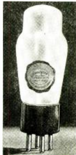
Battery-type ballast. (No. 463) This device eliminates rheostats.
