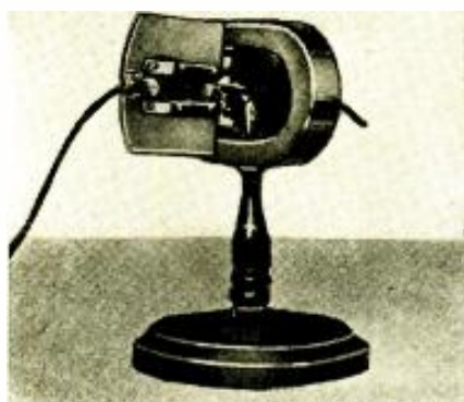
Fig. A Construction of "light gate."
