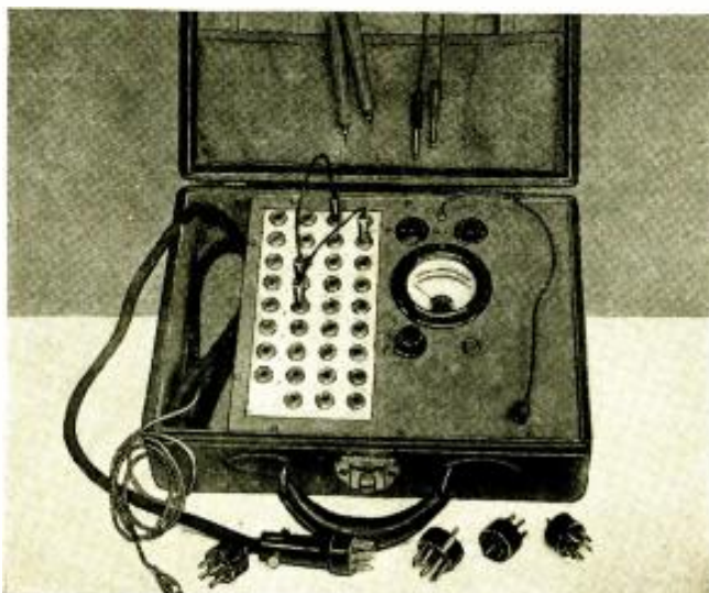
Fig. A Appearance of the analyzer. Note the amazing simplicity of this unit.
