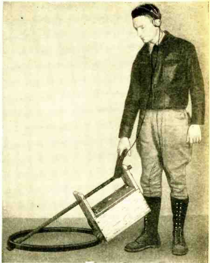
The device in the hands of the author. Note the distance between the ground and the loop.
