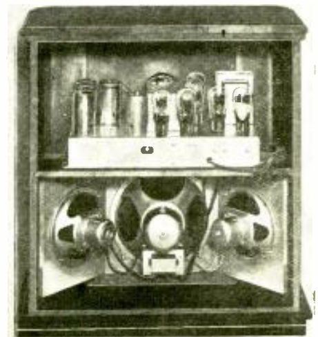
Photograph of the triple-speaker "Triolian" receiver.
