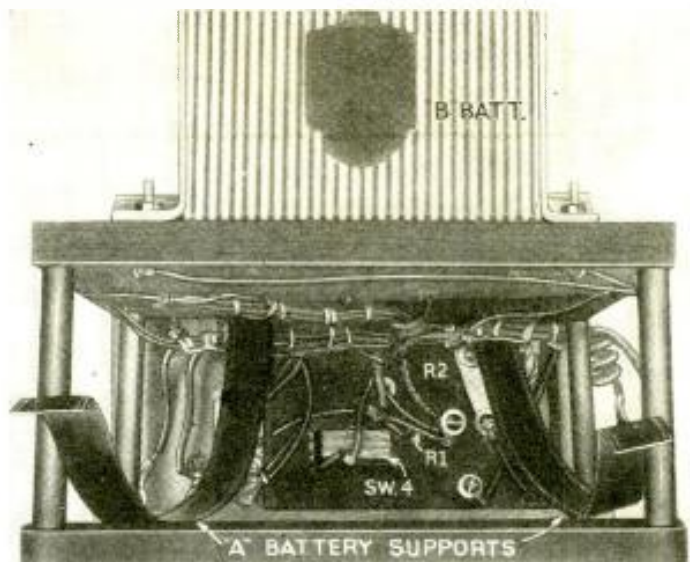
Fig. C A rear view. The two dry cells are placed alongside one another, from left to right, and are supported by the metal straps.
