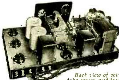
Back view of seven tube screen grid tuned Radio frequency receiver
