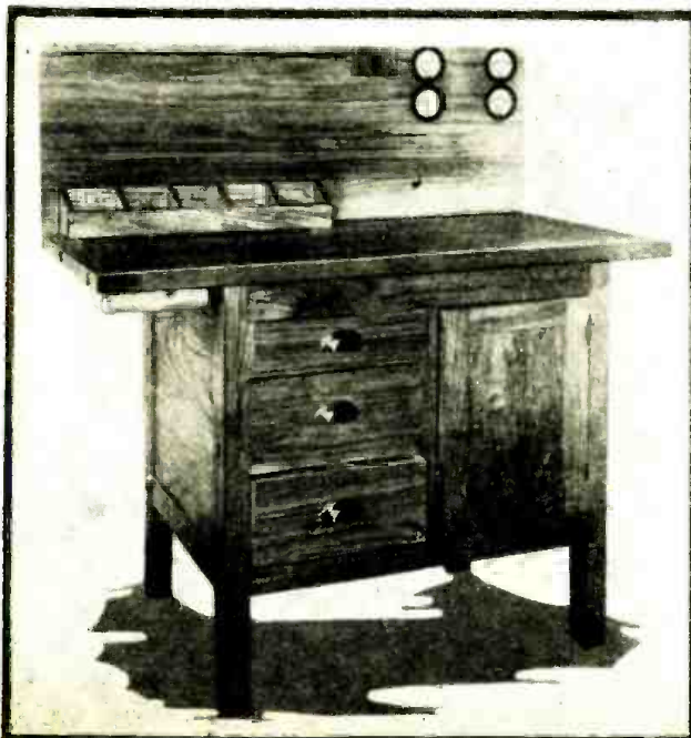
The work bench rearranged for the use of the Service Man; the radiotriician's tools replace the carpenter's. The Jewell meters shown are: one A.C. "Model 78," 0-3-15-150-volt reading; and three D.C. "Model 88" with these scales—0-15-150 ma. and 0-75-volt; 0-1-10-amp.; and 0-150-300-750-volt.
