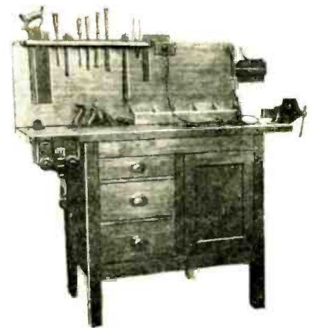
Mr. Weatherby's original design for the home mechanic. Everything is conveniently located, and the tools for wood and metal working are at hand.
