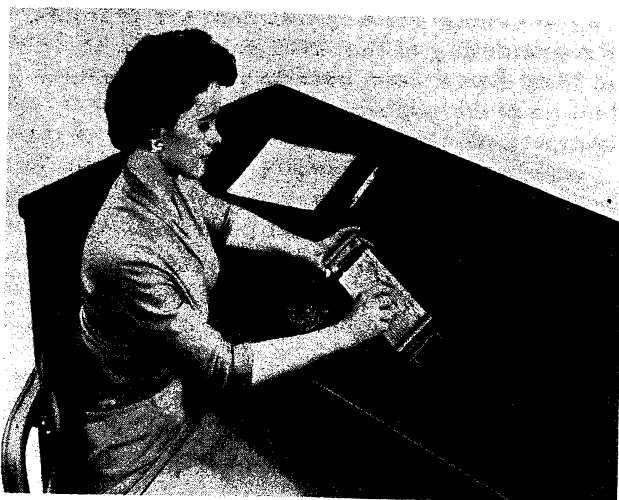
Fig. 2--Paper templates, marked with the proper pin positions, are laid over the pinboard, and the operator drops in the pins.
