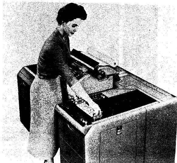
Fig. 3--Operator inserts an assembled pinboard. One problem may require as many as eight pinboards.
