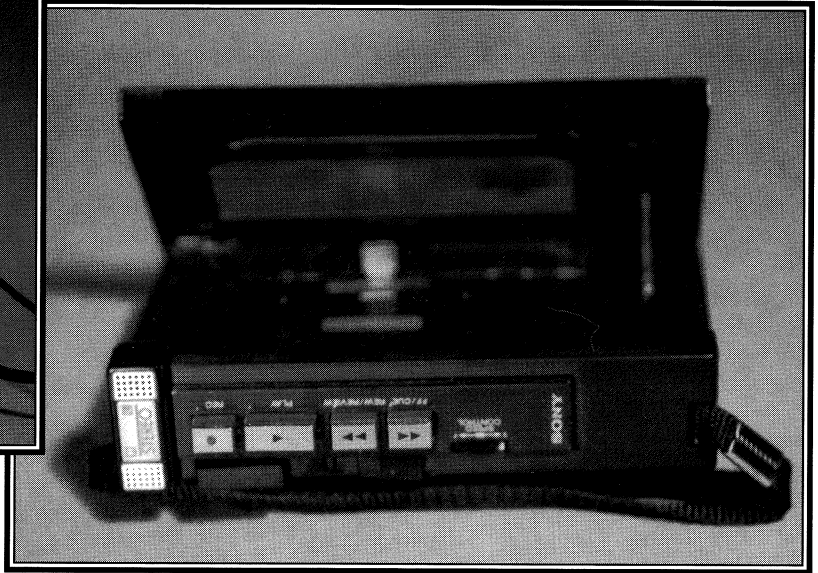
Sony binaural cassette tape recorder Model TCS-430. The space between the two mikes is about 3/4 inch.
