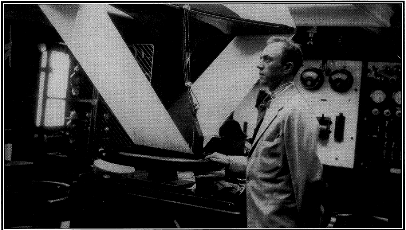
FIGURE 6. Paul Goodley at the VLF loop antenna aboard the Marconi yacht "Electra."
