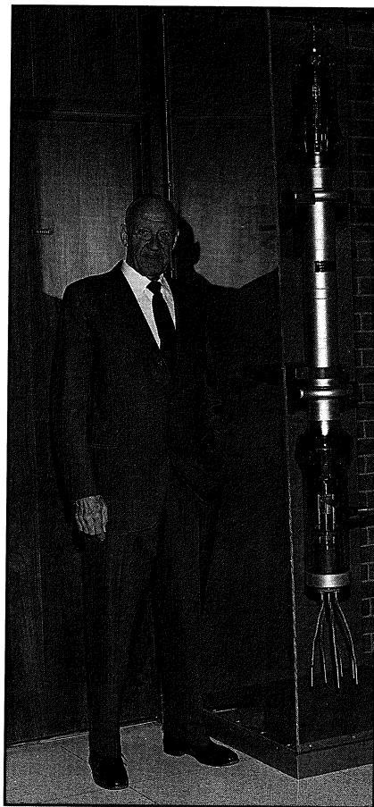
Figure 13. XERA designer, James O. Weldon, next to one of the 250 kw Western Electric 320A tubes at his company, Continental Electronics, in Dallas.
