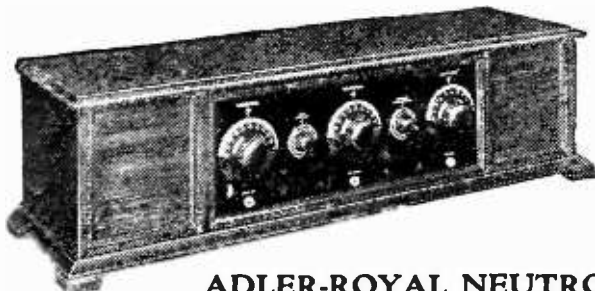
ADLER-ROYAL NEUTRODYNE Model 199 Table Type used with dry cells. Batteries concealed in cabinet. 5 tubes (199), Cabinets walnut or mahogany. Price $165.
