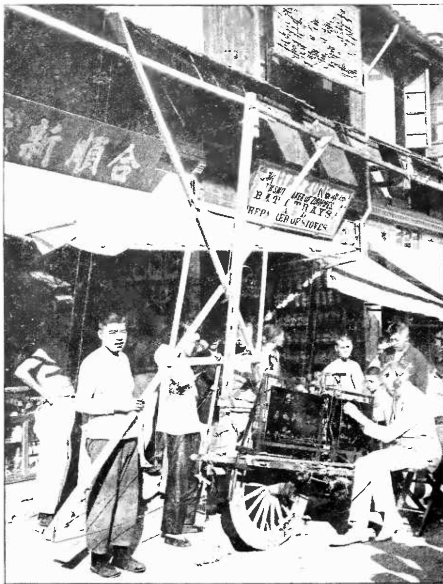
EXPERIMENTING WITH A LOOP TRANSMITTING AND RECEIVING STATION IN SHANGHAI
