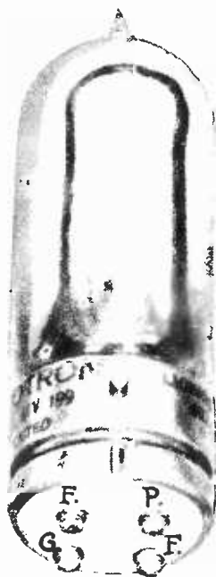
FIG. 3 Showing arrangement of contacts on the UV-199
