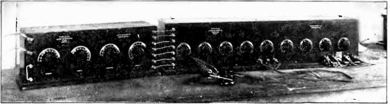
PANEL VIEW OF THE SUPER-HETERODYNE RECEIVING SET
