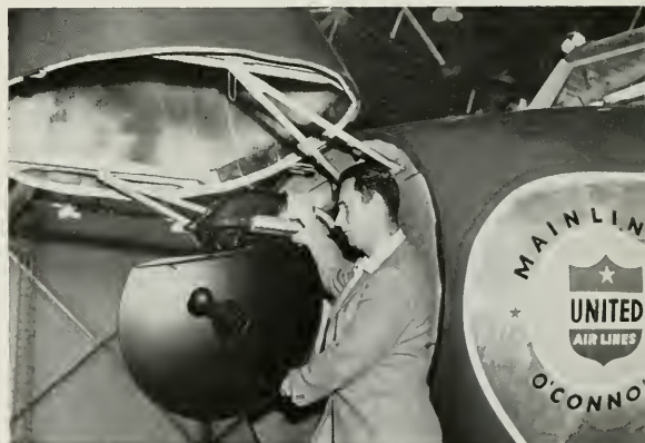
Nose of UAL Convair has been extended 28½ inches to house antenna and gear mechanism of RCA weather radar. Below, engineer checks radar installation in plane cockpit. Arrow indicates radar scope.
