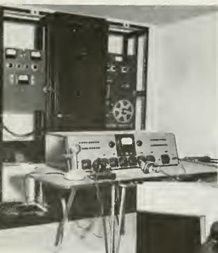
Photos taken before (left) and after (below) atomic blast show that RCA transmitter and associated equipment emerged with only minor damage.
