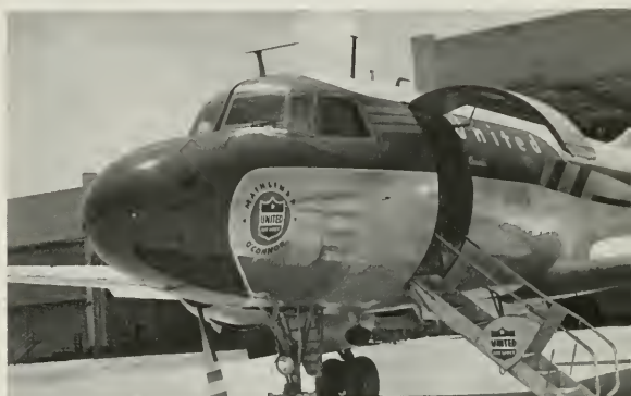
RCA weather radar is housed in nose of this UAL Convair executive plane.
