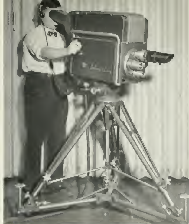
Improved model RCA Image Orthicon camera which provides brighter, sharper TV picture reception in the home.
