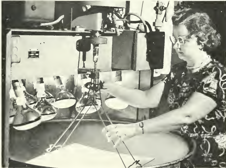
AN OPERATOR LOWERS A COPPER-CLAD SHEET OF PLASTIC, CONTAINING A PHOTOGRAPHIC PRINT OF THE TUNING CIRCUITS, INTO AN ETCHING VAT.
