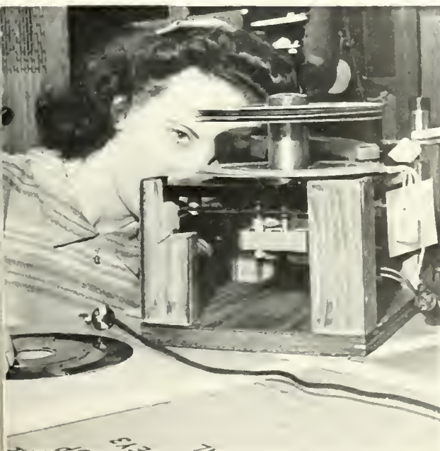
5 An inspector checks the operation of the disc-changing cycle of a record player.
