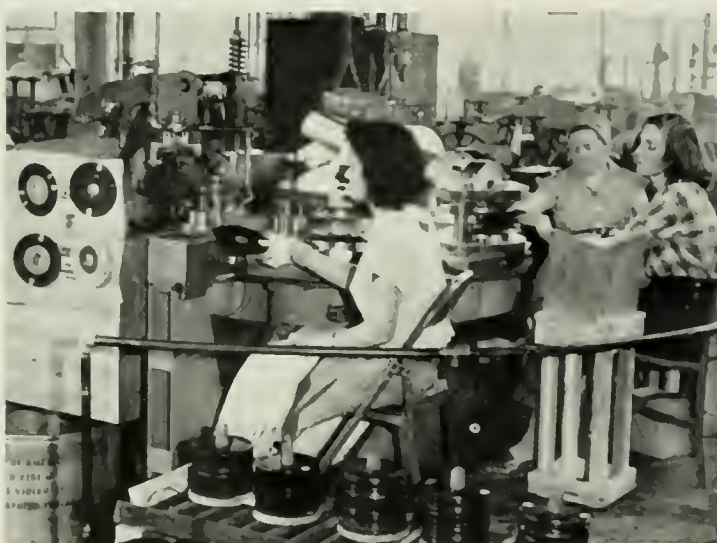
4 Each of these semi-automatic machines punches out the record's large center hole at the rate of 30 discs a minute.
