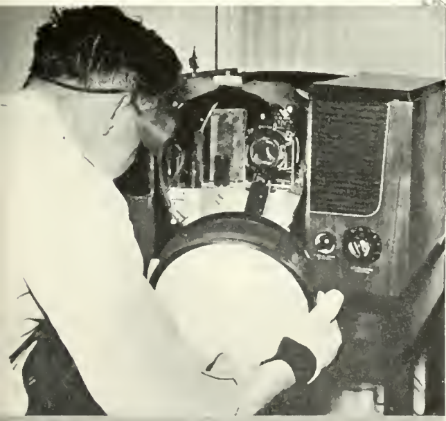
7. A 10-inch RCA kinescope is inserted into the socket of the television receiver to complete the installation inside the home.
