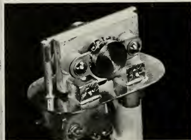
THE TYPE 2J41 MAGNETRON WAS THE FIRST TO HAVE ITS FREQUENCY STABILIZED BY AN EXTERNAL CAVITY DISTINCT FROM THE CAVITIES WITHIN THE TUBE.
