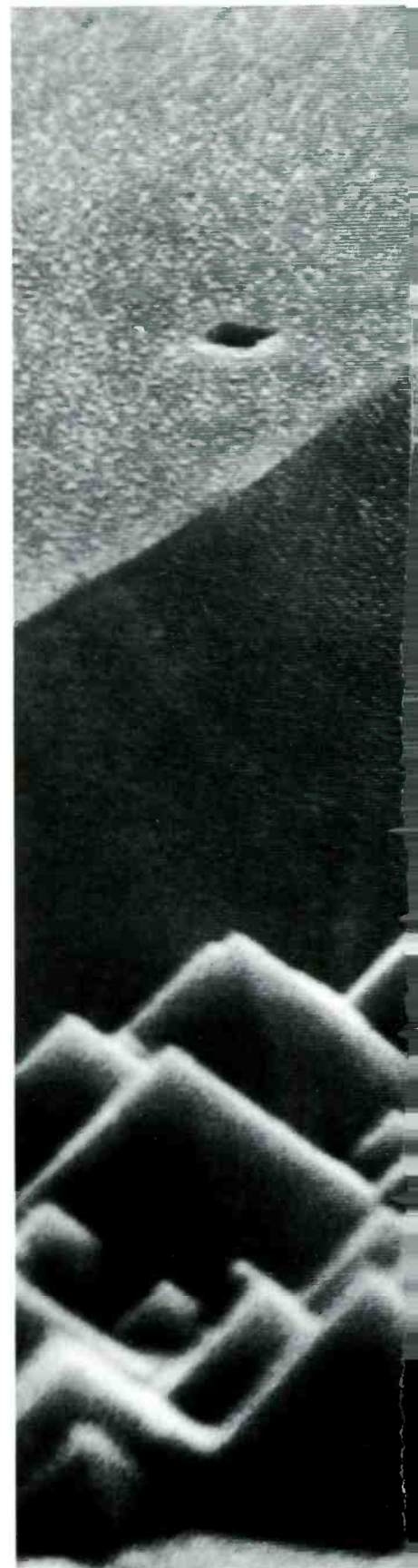
Electronically active surfaces seen through a scanning electron microscope: top, spontaneous growth of germanium whiskers, magnified 6,000 times; left, pressed zinc oxide powder magnified 3,500 times; right, crystals of silicon—magnified 8,000 times—grown on a sapphire surface.
