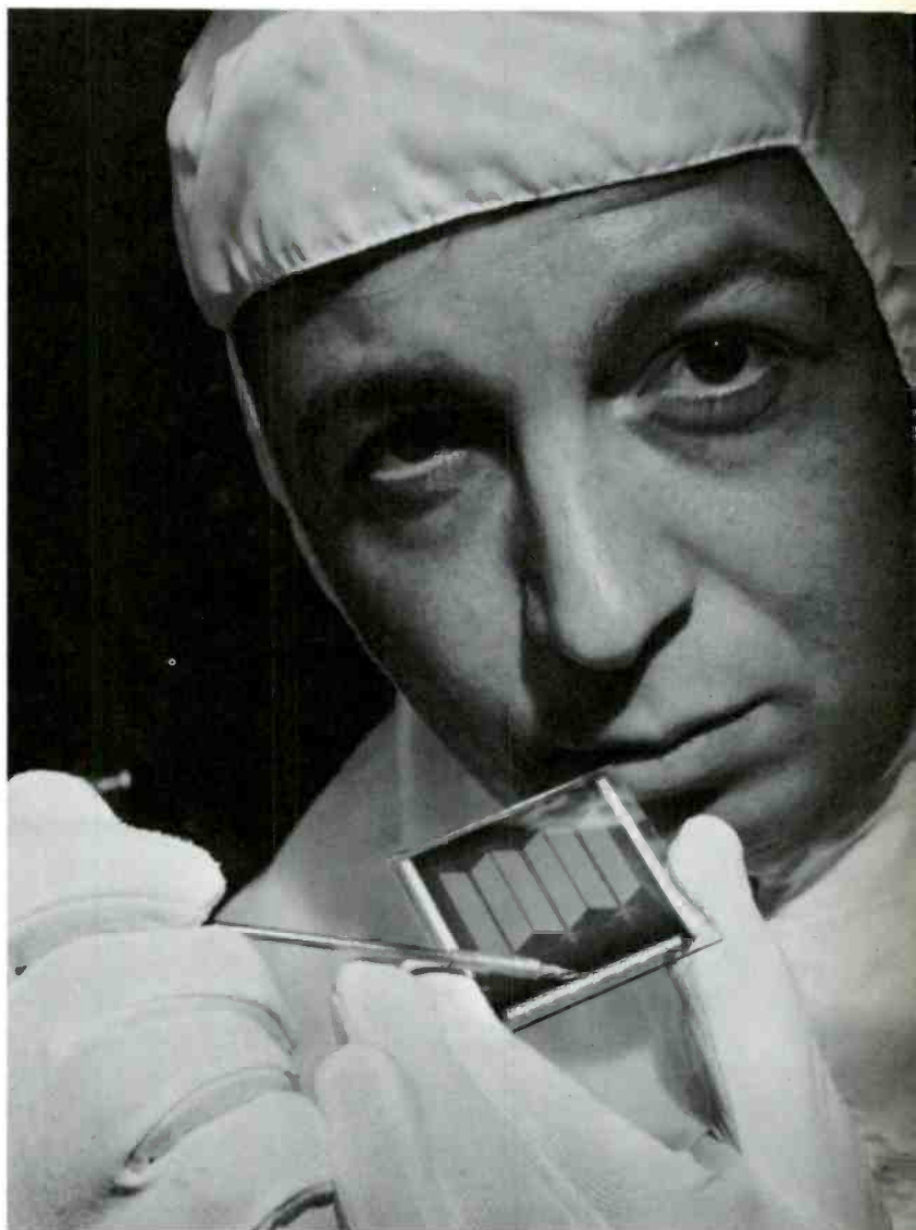
An experimental superconductive computer memory, which in its final form will be capable of storing 250,000 bits of information, is held by Robert Gange. Memory is kept at liquid helium temperature.
