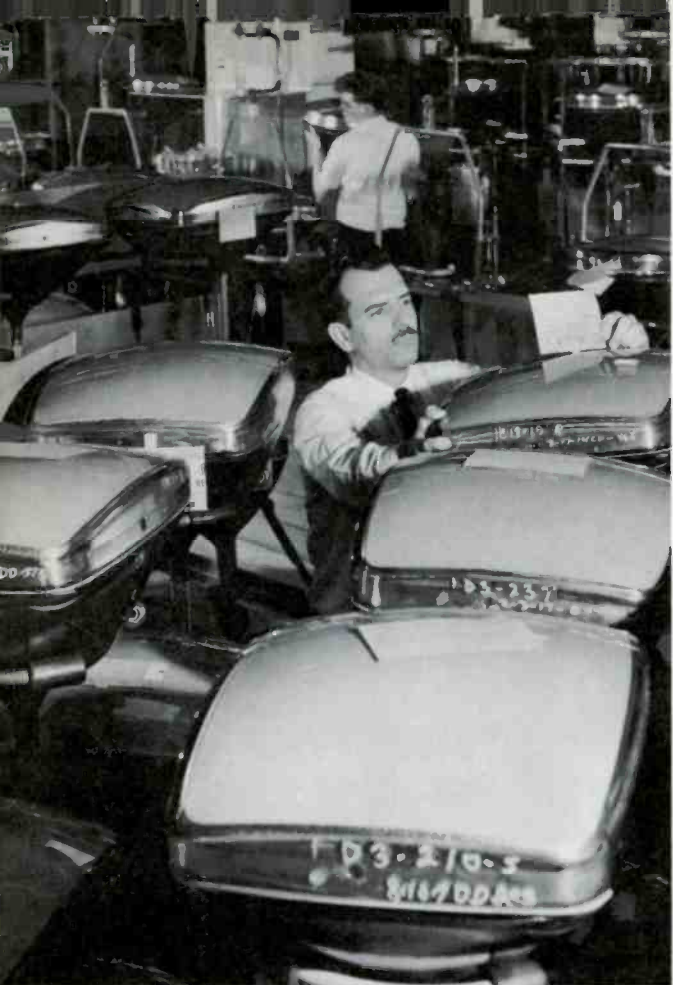
Production of 25-inch rectangular color TV picture tubes at RCA plant in Lancaster, Pa.
