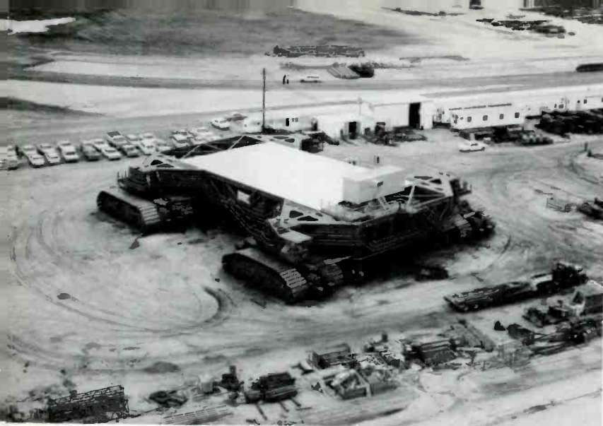
The Crawler-Transporter, world's largest land machine, will haul the Saturn 5/Apollo and the Mobile Launcher from the assembly point to the launch site.
