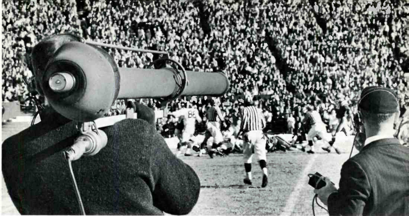
This directional microphone allows the viewer to hear the play of the game.
