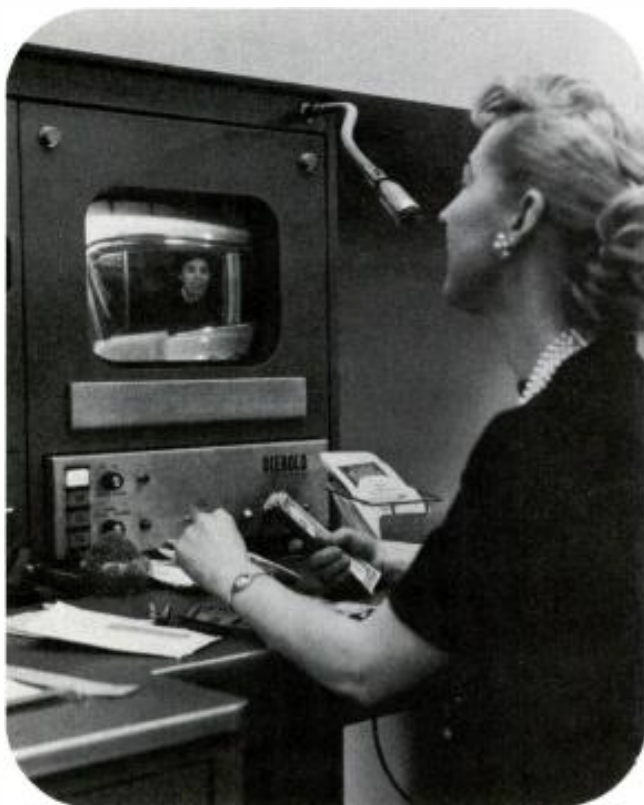
Teller's Eye View: Hundreds of feet apart, teller completes bank transaction over closed-circuit TV with customer.
