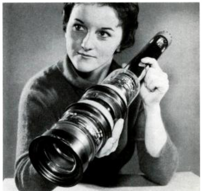
Image intensifier orthicon electron tube makes it possible to photograph stars millions of times dimmer than the naked eye can see.
