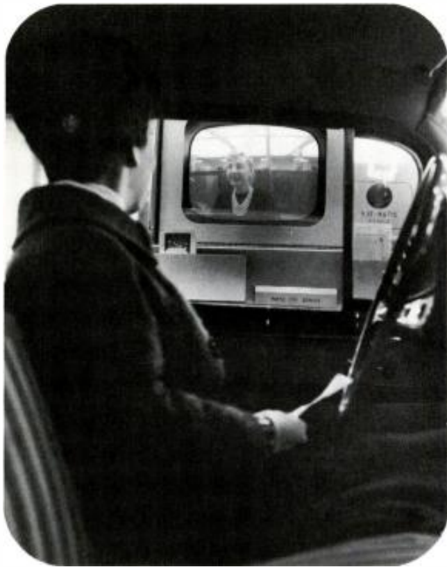
Customer's Eye View: Out-of-doors, customer in auto sees teller inside the bank on TV monitor and converses over two-way voice circuit.
