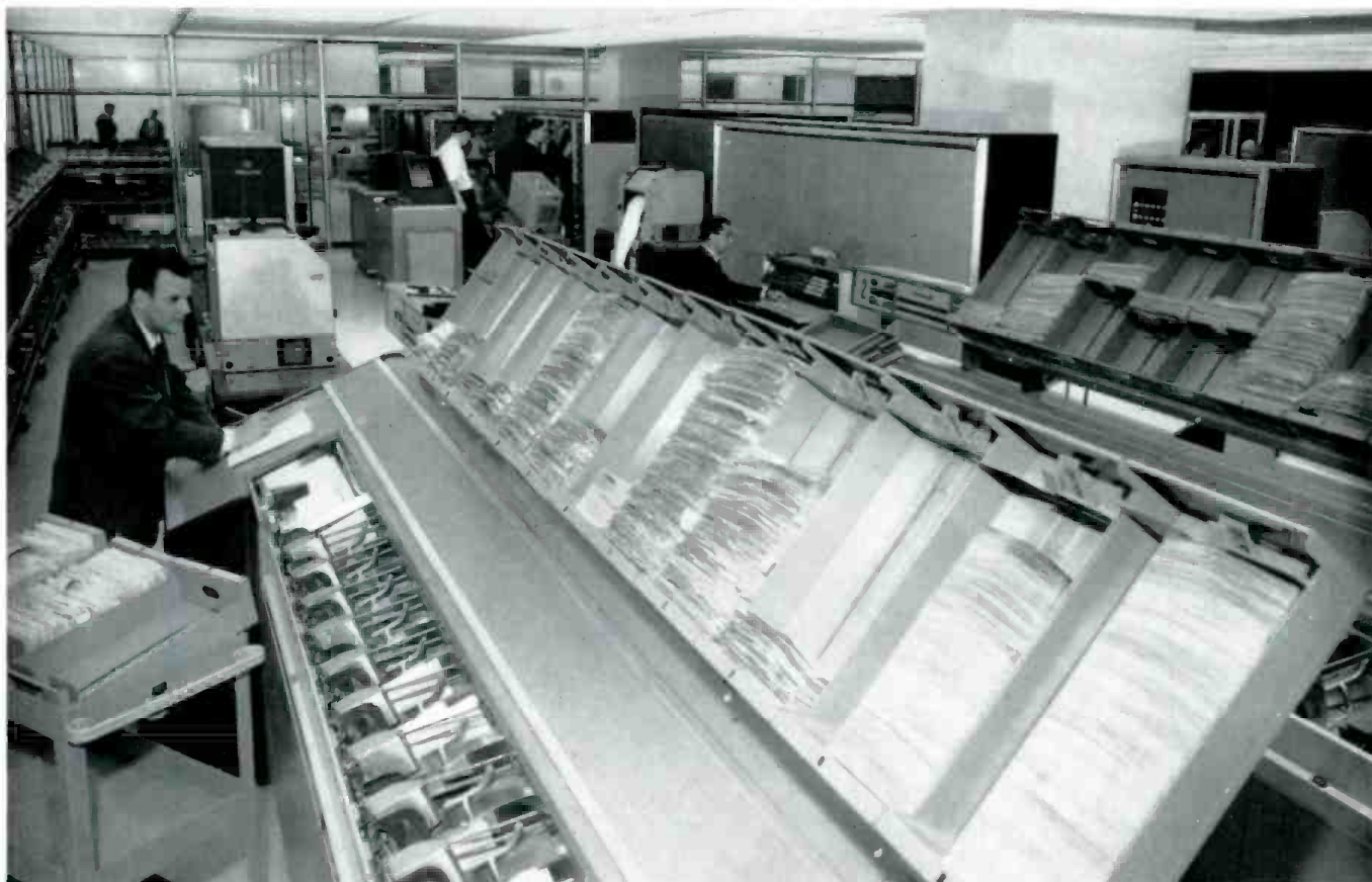
An electronic check sorter, one of seven, reads each check and feeds information to RCA 301 systems for conversion to magnetic tape.
