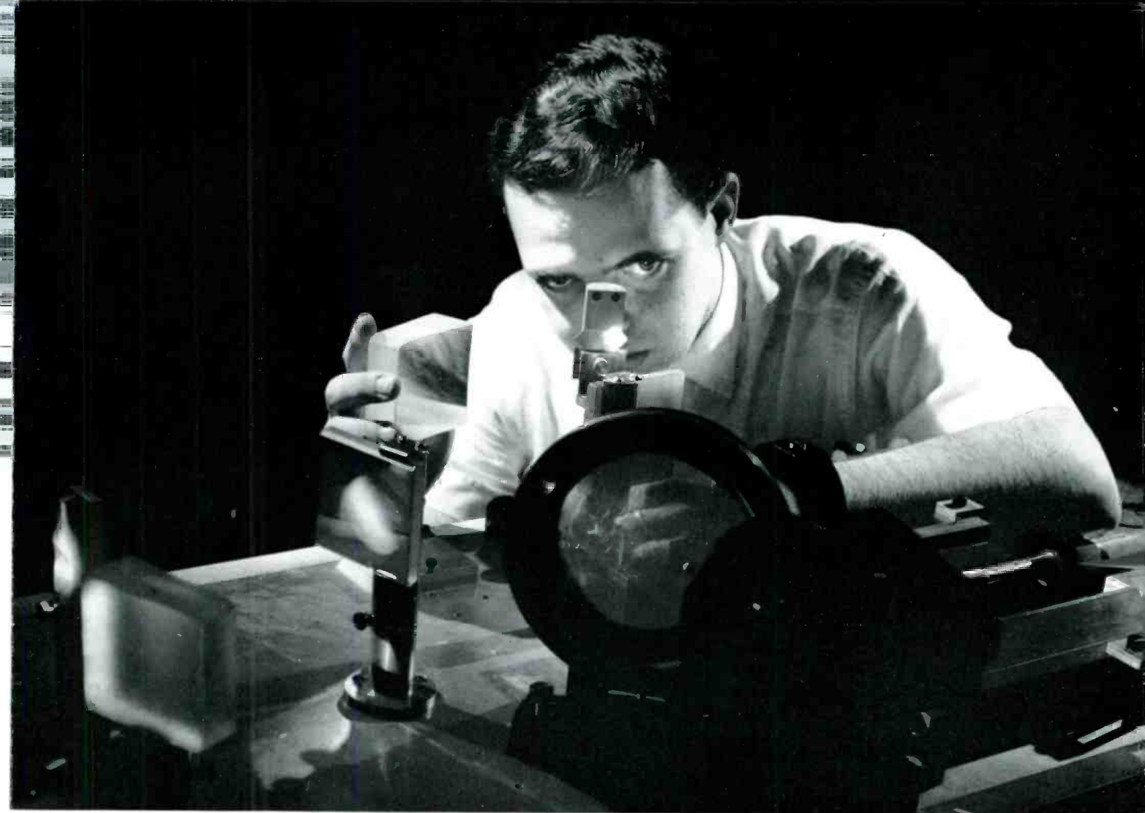
John McCormack prepares to analyze the frequencies of a laser beam with a new interferometer built by RCA scientists in Princeton.
