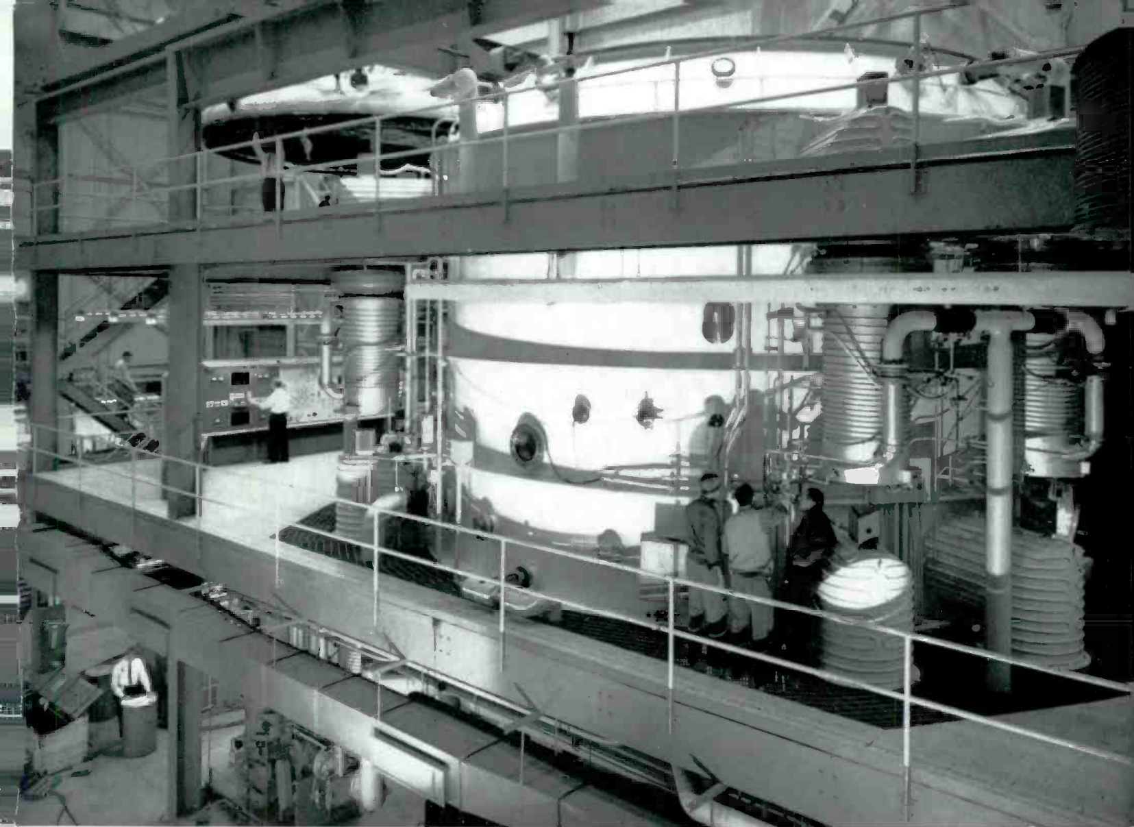
Completed spacecraft can be tested before flight in this large thermal vacuum chamber at RCA's new Space Environmental Test Center.
