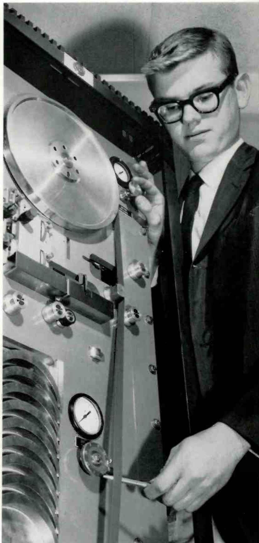
A developmental High Speed Tape Loop for gathering and recording data in military systems is put through a test.
