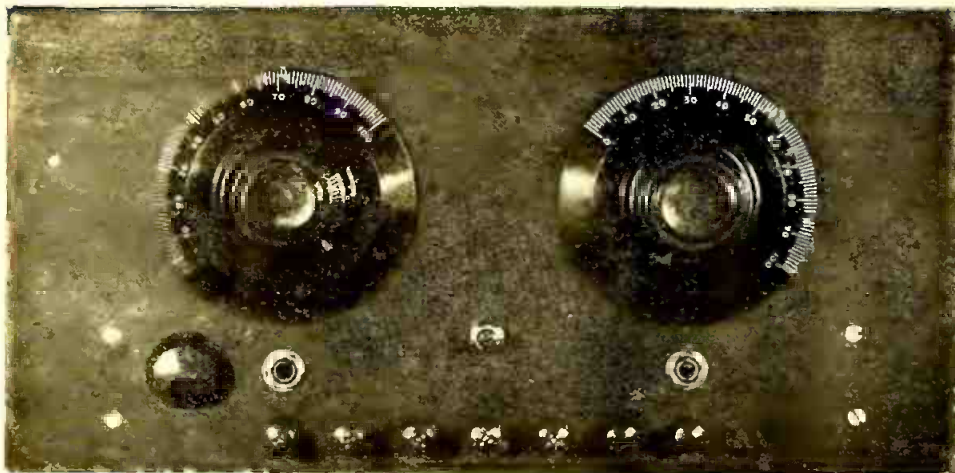
Front panel view of the completed short wave receiver. The dial to the left is the wavelength control, while the one on the right controls the tickler or regeneration coil.
