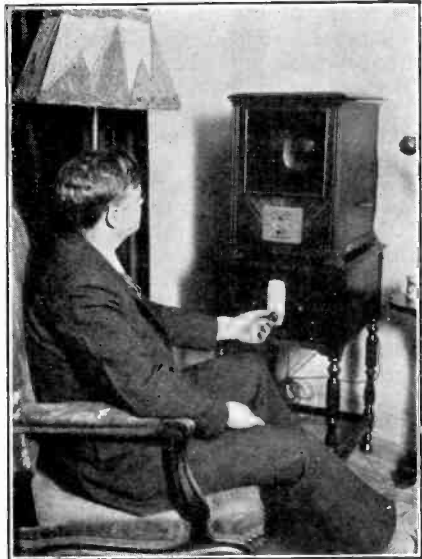
A Jenkins Model 200 Radiovisor in the home. The front of the cabinet contains a shadowbox leading to a large recessed magnifying lens through which the radiovision images are viewed in enlarged form.
