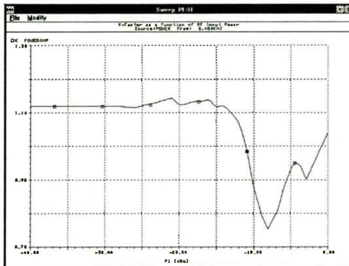
Figure 15(a) Stability Factor of Amplifier at 450 MHz as a function of RF Input Power
