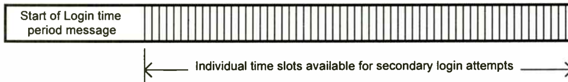
Fig 4.2 A start of login time period message followed by ALOHA login time slots.
