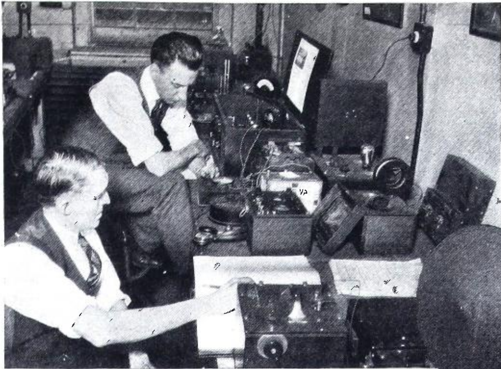
Experts in the POPULAR RADIO Laboratory with measuring apparatus arranged for loudspeaker tests.
