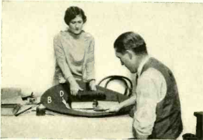
7 After the circle, O, in cone B has been cut out, the two back rings, C and D, should be carefully centered over the hole that is left and cemented to either side of the disc. Two or three heavy books should then be laid on ring D until the cement has hardened.
