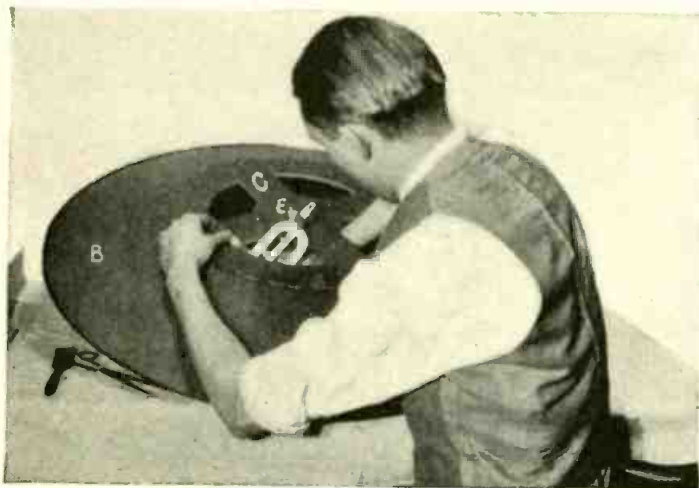
9 The loudspeaker unit, E, is inserted through the back rings, C and D, to which it is fastened by means of three brackets and bolts. The brackets, of course, should be fastened to the rings before the unit is inserted.
