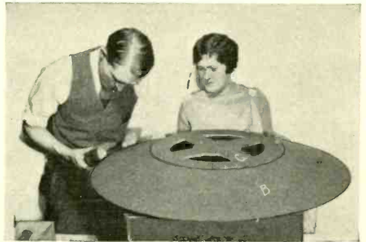
8 To cement the two discs together, disc A is set in a support, as shown in Figure 4, and disc B is set carefully into it. The cement is then evenly poured around the rim of disc B at the point where the two cones meet; this fastens the cones together solidly.
