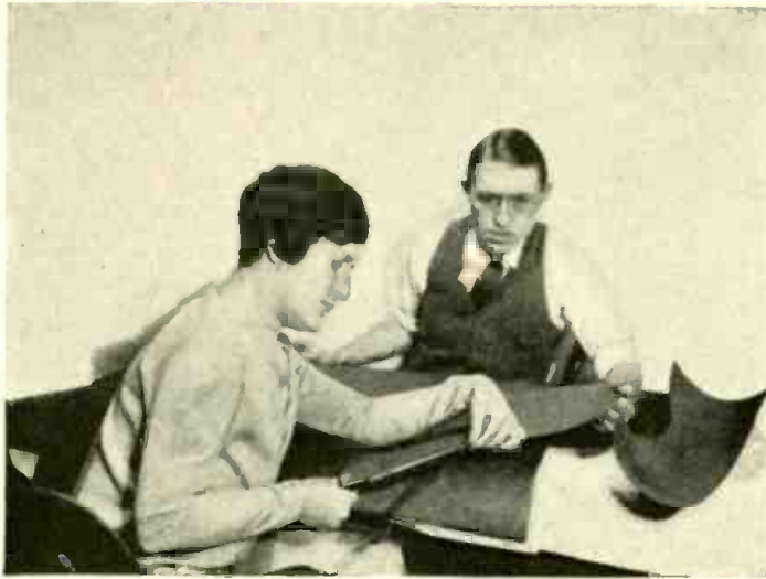
5 After the cone paper has been marked in pencil, as shown in Figures 1 and 2, the two discs, A and B, should be cut out carefully with a sharp pair of scissors, and the segment cut out between lines 1 and 2 (of the diagrams).
