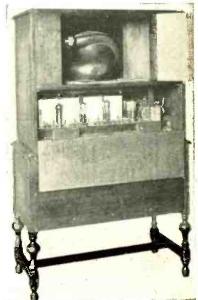
The rear view of the Kellogg receiver showing the set assembly with the tubes in place and the loudspeaker installed in the upper portion of the cabinet.
