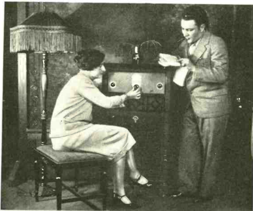
This new Stewart-Warner receiver, unlike most single-control sets, has no auxiliary or balancing controls; all the tuning is done with the knob in the center of the panel. The left-hand control is connected in the plate circuit of the radio-frequency tubes and may be used to adjust the volume; the right-hand control regulates the amount of filament current fed to all the tubes and requires no attention.
