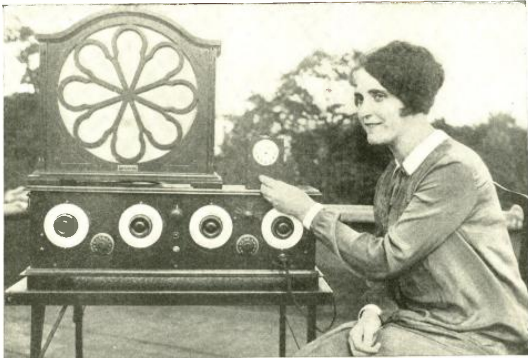
HOW THE CLOCK IS "SET" TO CONTROL THE RECEIVER It is connected up to the batteries that feed the receiver, and by a contact of one of the moving parts turns the receiver "on" and "off" at the time to which the clock is regulated.
