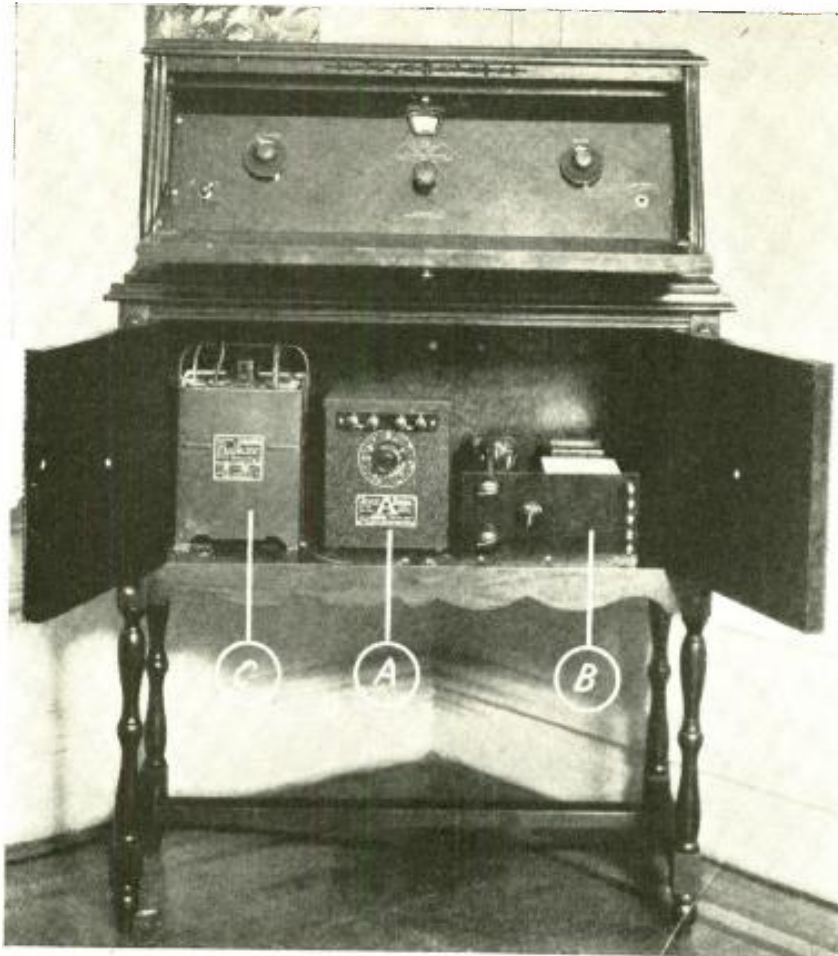
THE "A" AND "B" POWER-PACKS INSTALLED
