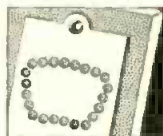
Screw Template to panel.
