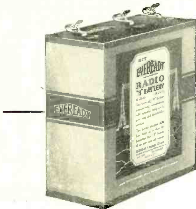
Eveready "B" Battery No. 772 for detector and amplifier. Connections at 22½ and 45 volts. Three Fahnestock Clips. Approximate over-all dimensions, 8¾ in. x 3¾ in. x 7¾ in.
