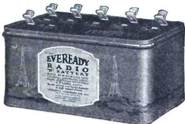
Eveready "B" Battery No. 766. 22½ volts. Six Fahnestock Spring Clip Terminals, giving variable voltage from 16½ to 22½ volts, in 1½-volt steps. Length, 6¾ ins.; width, 4¾ ins.; height, 3 3/16 ins. Weight, 5 lbs.
