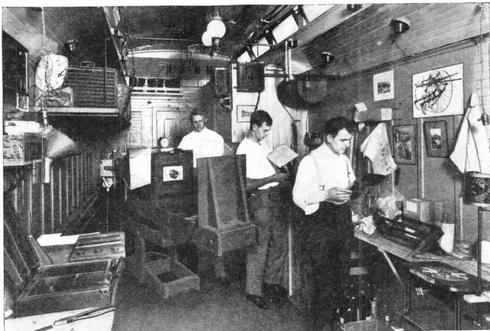
A Complete Engraving Plant on a Railroad Car — Making the Plates for Illustrations
