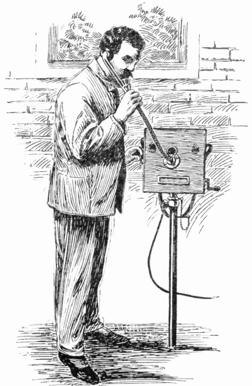
Telephone Test Set
