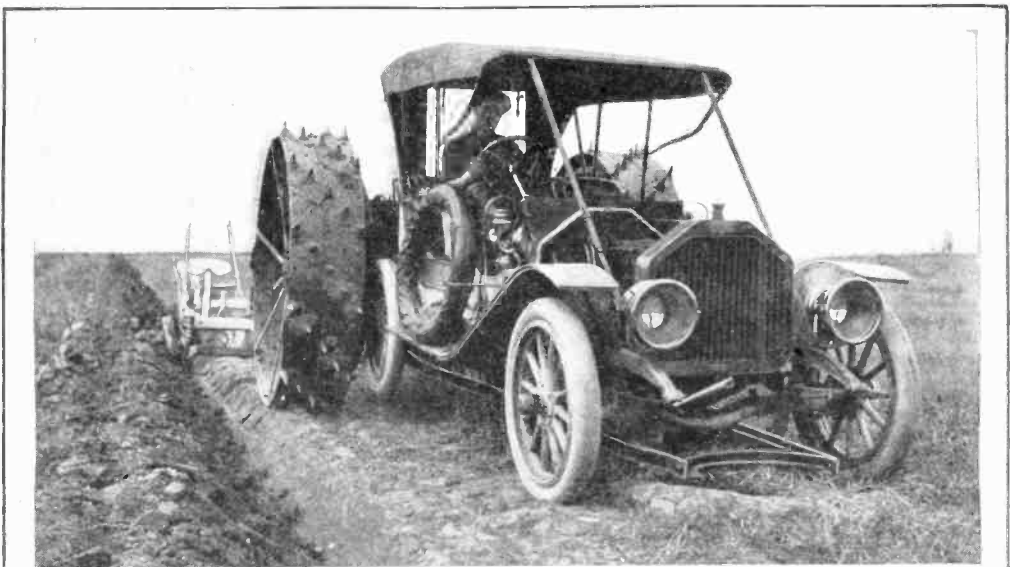
Two Machines in One. In Five Minutes the Automobile may be Attached to or Detached from the Tractor
