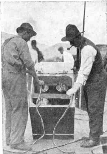
UNPACKING ARC LIGHTS, SHOWING THE STANDARD CASE IN WHICH THEY ARE TRANSPORTED
