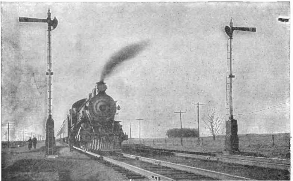
FIG. 19. LOS ANGELES LIMITED NEAR KEARNEY, NEBRASKA, OBEYING A "STOP"
