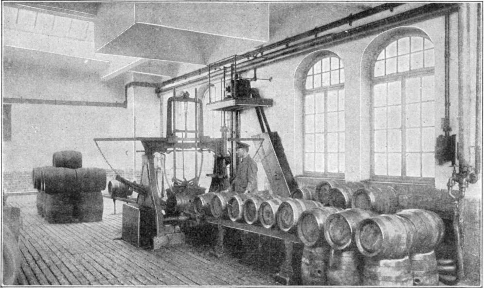
ELECTRICALLY DRIVEN MACHINE WHICH WASHES KEGS AND BARRELS
