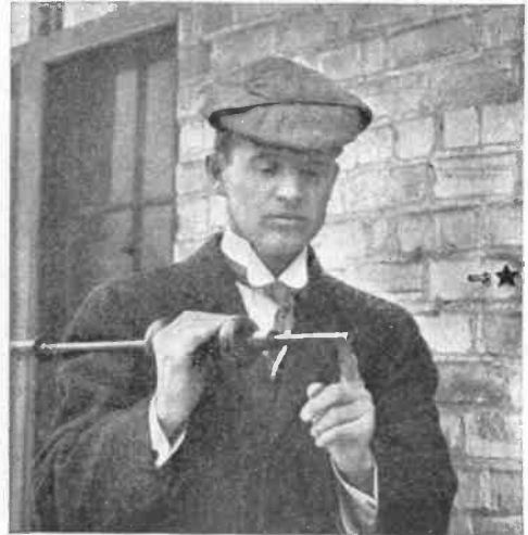
THE REVERSE END OF THE HAMMER-DRIVE IS A HOLLOW PUNCH WHICH SLIPS OVER THE BOLT. FIVE BLOWS OF THE SLIDING HAMMER DRIVE IT HOME
