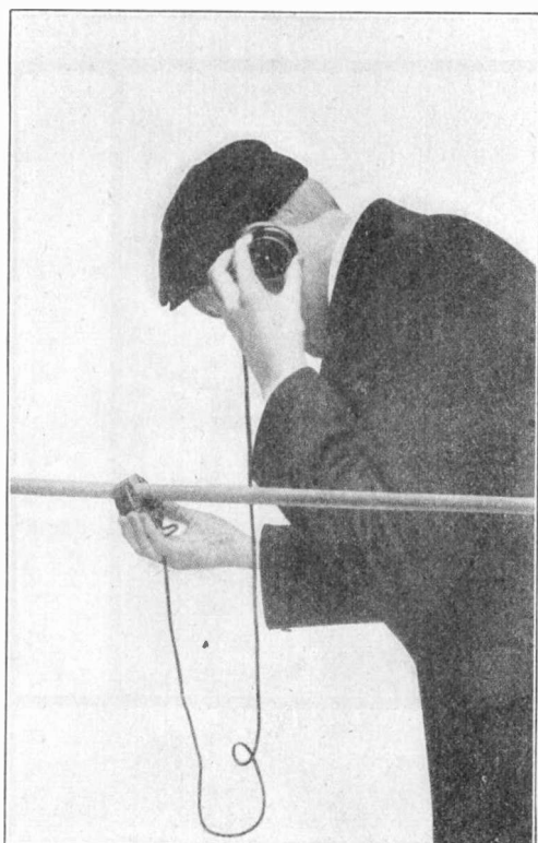
FIG. 1. DETECTING CURRENT BY MEANS OF A TELEPHONE
