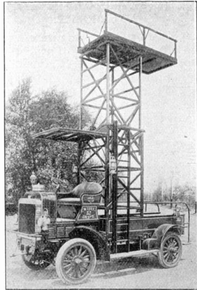
"TROUBLE" WAGON WITH PLATFORM RAISED READY FOR WORK.
